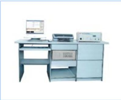
Automatic measurement on basic magnetization curve and magnetic hysteresis loop under static state of soft magnetic material, accurate measurement on static magnetic characteristic parameters such as initial permeability  $\mu_i$ , maximum permeability  $\mu_m$ , saturation magnetic induction  $B_s$ , remanence  $B_r$ , coercive  $H_c$  and hysteresis losses  $P_u$ .
