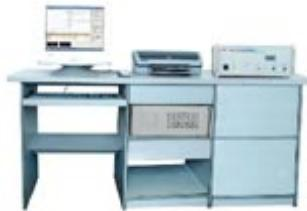
Automatic measurement on basic magnetization curve and magnetic hysteresis loop under static state of soft magnetic material, accurate measurement on static magnetic characteristic parameters such as initial permeability  $\mu_i$ , maximum permeability  $\mu_m$ , saturation magnetic induction  $B_s$ , remanence  $B_r$ , coercive  $H_c$  and hysteresis losses  $P_u$ .
